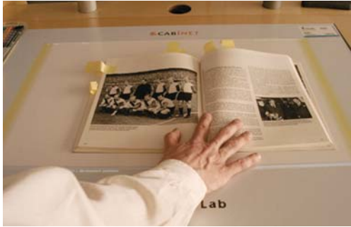
FIG. 09 Interaction with Cabinet. Upper row: adding physical material by laying a magazine, book or object on the table. The material is photographed from above and projected in place. Lower row: interacting with thumbnails and grouping thumbnails on stacks
